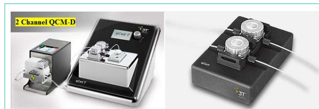
Figure 1: Exemplary acoustic (QCM-D) instrument (www.3t-analytik.de).
