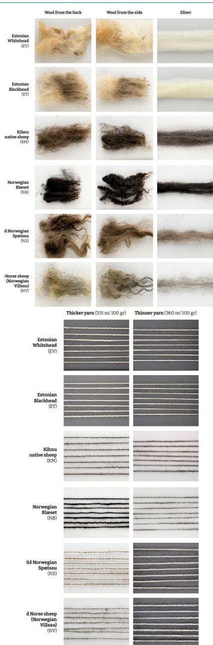
Figure 7: Samples of wool, sliver and yarn of six sheep breeds. Order from left: wool from the back, wool from the side, sliver, thicker yarn (315 m/ 100 gr), thinner yarn (360 m/ 100 gr). Photos by Maritta Anton.
