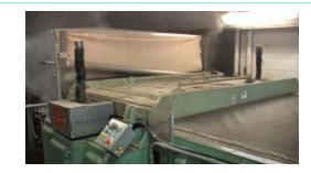
Figure 2: Oscillating plate and steam apply.
