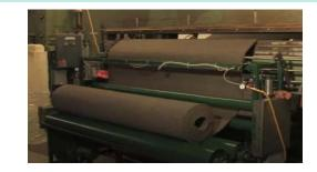
Figure 3: Final product (felt) in roll form.
