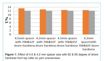
hardness on the yarn unevenness is plotted in (Figure 1). The spacer of 4.2mm with 62 degrees of shore hardness gives the best even yarn with a low u% of 35.5Nm. In the case of smaller spacer sizes there is better control of short fibers. Evenness is improved by closing down the apron spacing.
