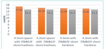
Figure 2: Effect of 4.5 & 4.2 mm spacer size with 62 & 65 degree of shore hardness front top roller on yarn coefficient.
