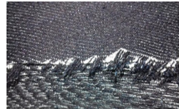
Figure 12: Spandex breakage due to cutting of fabric.
