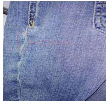
Figure 11: Spandex breakage in the sewing line.
