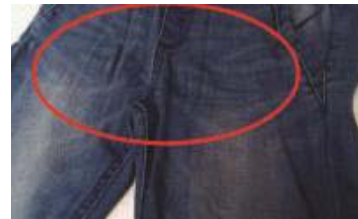
Figure 18: Spandex breakage due to incorrect mechanism and machine setting.
