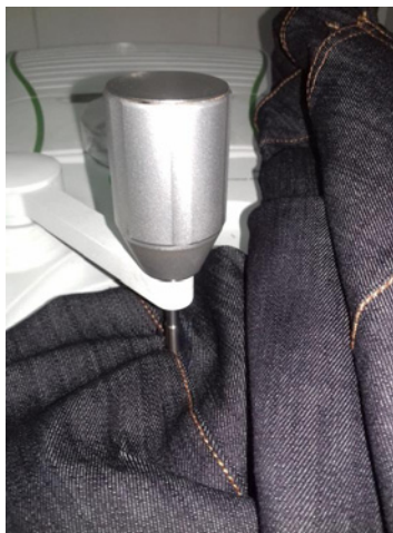
Figure 20: FTIR experiment on the garments of no spandex breakage.
