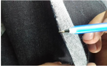
Figure 13: Spandex is going inside due to cutting finding no tension.
