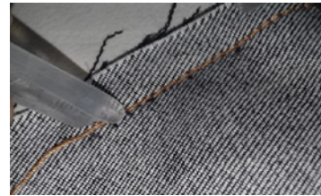
Figure 17: More stitch per inch damages more spandex in the fabric.
