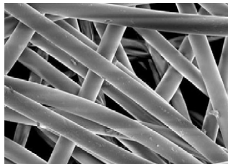
Figure 2: Scanning Electron Microscopic View of polypropylene fibers.
