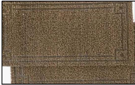
Figure 4: Jute polypropylene composite plate produced by molding with hot pressing.
