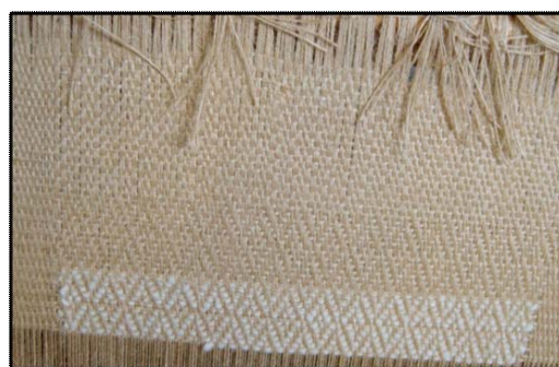
Figure 3: Woven fabric was made by jute (warp) yarn and polypropylene (weft) yarn.
