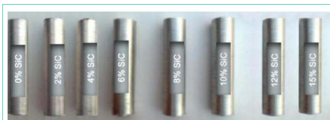
Figure 2: AL/SiC metal matrix composites fabricated by Stir Casting method [12].
