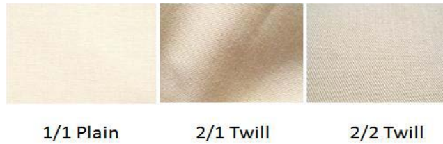
Figure 1: 1/1 plain, 2/1 Twill, 2/2 Twill fabric has been taken from the test specimen.
