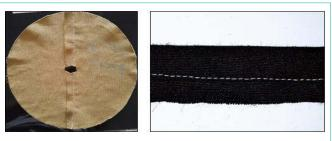
Figure 1: Sample preparation for drape coefficient and stiffness.
