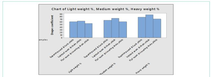
Figure 12: Drape coefficient of different seamed fabric with stitches.
