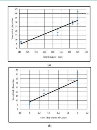
Figure 6 (a, b): Yarn number of thick places/km versus fiber fineness,  ${\rm SFC}(n)\%$
