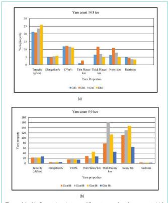
Figure 1 (a, b): Comparison between different properties of yarn counts14.8 and 5.91 *tex.*
