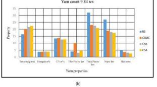
Figure 12 (a, b): Yarn properties of different systems - RS, CSA, CSB, and CSMC.
