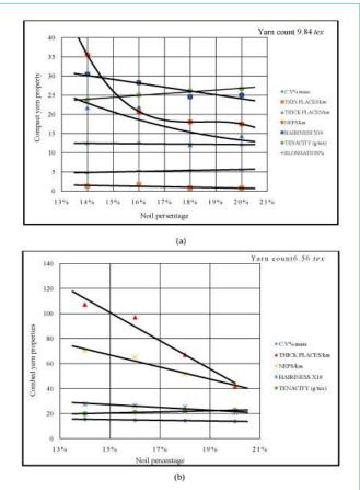
Figure 11 (a, b): Compact yarns properties versus the noil percentage for count 9.84 and 6.56 *tex*.
