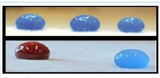
Figure 1: Photographs of droplets of water on treated cotton (above) and droplets of water and olive oil on treated silk (below). For demonstration purposes water and oil were enriched with a blue and a red pigment, respectively.
