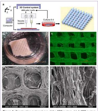
**Figure 1:** Construction and analyses of the 3DP system. (a) A 3DP system extruding ADSCs loaded gelatin/alginate/fibrin hydrogel in grid structure. (b) The 3D structure cultured in a plate. (c) Immunofluorescence staining of the 3D construct with mAb against CD34+ (in green). (d)-(e) Scanning electron micrographs (SEM) showed the development of extensive ECM and cell networks in the construct after 6 days of engagement [26,27].
