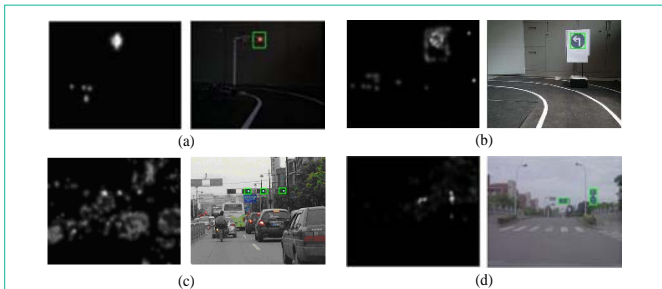
Figure 6: Traffic light and traffic sign detection result, (a) and (b) are in micro traffic environment, (c) and (d) are in actual traffic environment, with CSM image (left) and detection result (right).
