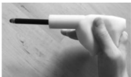
Figure 3: 3D-Printed Grip with Stylus [17] (adapted and modified).
