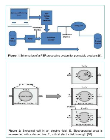
power supply, energy storage capacity, and computer for operating the system controls. A continuous flow diagram for PEF processing is illustrated in Figure 1.
