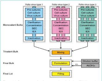
**Figure 1.1: Process overview for preparation of trivalent IPV**. Monovalent bulks are prepared for each poliovirus (type 1, 2 and 3) separately. Virus was harvested, clarified, concentrated, and purified, first on size using Size Exclusion Chromatography (SEC) and Ion Exchange Chromatography (IEX). Purified virus were mixed with buffers and Aluminium Hydroxide Al(OH)<sub>3</sub> prior to filling [1].
