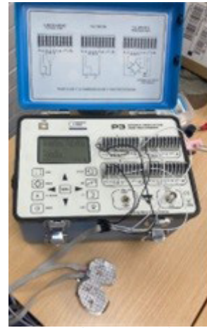
Figure 21: Sensor connected to strain indicator.
