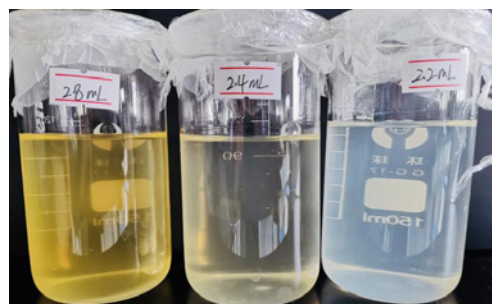
Figure 2: Effect of ammonia dosage on the color and transparency of Hp55S glue (50°C).
