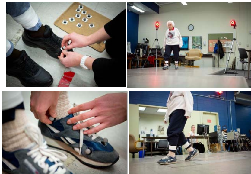
Figure 2: Reflective markers attached to shoes to capture motion for gait analysis.
