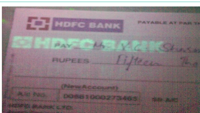
Figure 6: Specimen Cheque 2: Chemical Watermarks appear as "HDFC BANK" under UV light.
