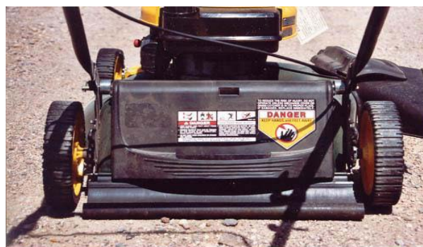
Figure 8: The discharge door of the mower appears securely in place with no gaps or defects and the trail guard is in good condition.
