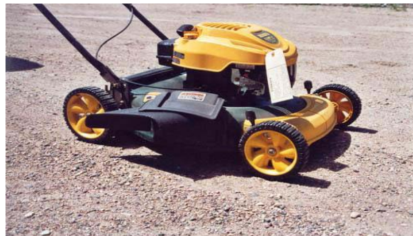
Figure 7: Examination of the lawn mower revealed the mower to be in good working condition with no safety modifications noted. The mulcher door was up with an attached discharge guard which appeared securely in place.
