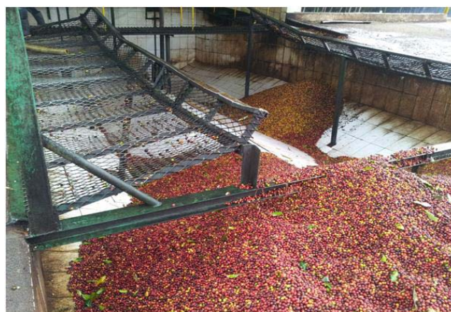
Figure 1: A small scale wet processing set-up (Santa Sofia) for coffee beans with the location in Aldea Ayarza, Casillas Santa Rosa, Guatemala.
