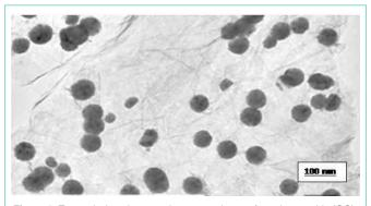
Figure 1: Transmission electron microscope picture of graphene oxide (GO). Diameter size 38nm.
