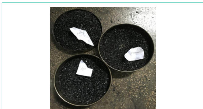
Figure 3: Coal sample with initial particle size of 4~7 mm.
