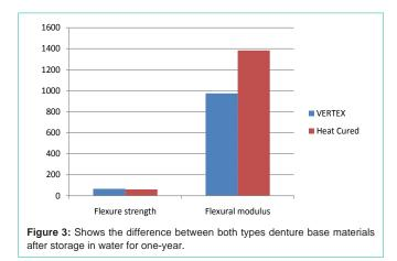
using Instron Universal Testing Machine (Instron, USA.) with load cell 500 N Bluehill Lite software at cross head speed 1mm\min. The maximum load for fracture was recorded in (N) and the deflection of the specimens at fracture was recorded in mm. For calculating the flexural strength in MPa, the following formula was used: Stress =  $3 \times \text{Load} \times \text{Length} / (2 \times \text{Width} \times \text{Thickness}^2)$  [16,17]
