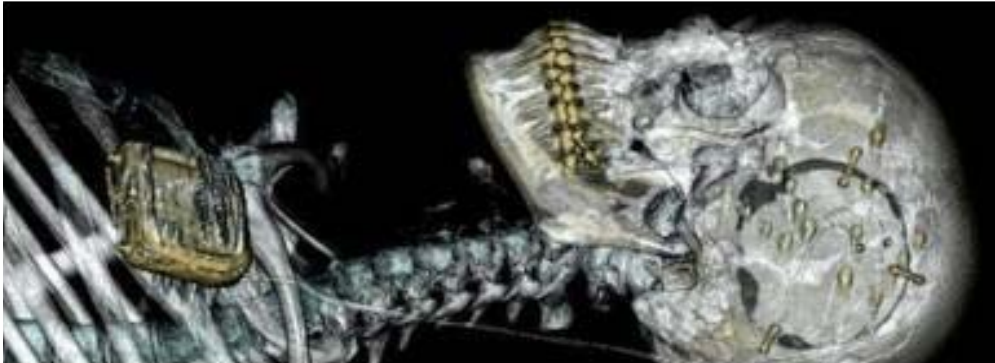
Figure 1: CT scan of the NeuroVista seizure advisory system implanted in a patient [8].
