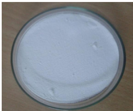
Figure 1: KOH supported on alumina catalyst used for transesterification reaction.
