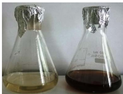
Figure 1: Control (left) and silver (right) nanoparticles synthesized from Epiphyllum oxypetalum .
