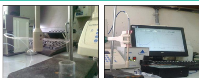
Figure 1: (A) Fitting of microchannel within fiber optics dip probe (B) Assembly of the System.
