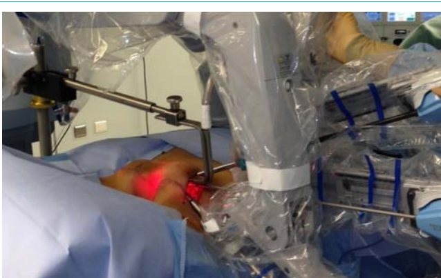
Figure 2: Placement of the retractor and Da Vinci Si HD robot arms in position during console working time.
