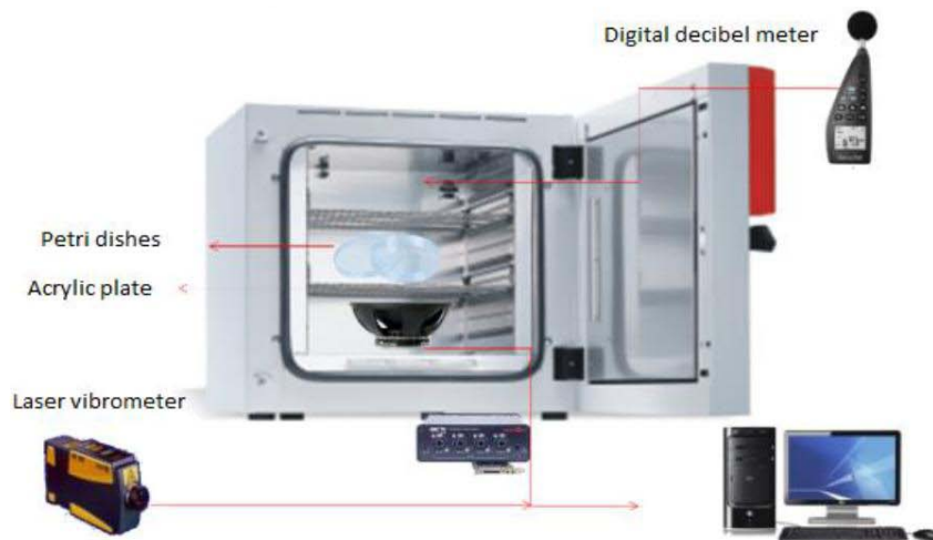
Figure 1: Schematic sound wave load apparatus. Sound wave apparatus adapted to an oven to produce an environmental sound stress.
