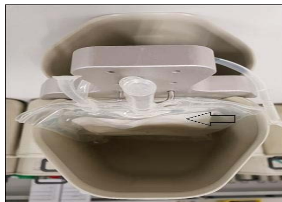
Figure 2: The support. A support (indicated by the arrow) was added to the centrifuge insert. This enabled the unit and its components to keep steady throughout the centrifugation process.
