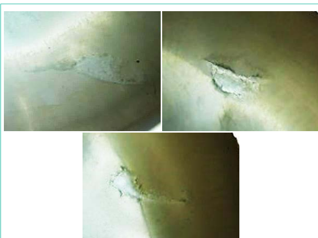
Figure 11: Optical microscope images of the crater in enamel by using energy densities of 17.08, 11.18, and 5.6 J/cm 2 .
