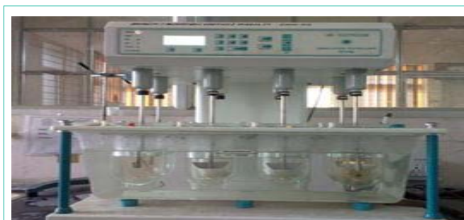
Figure 2: Assembly for In-vitro drug release studies.
