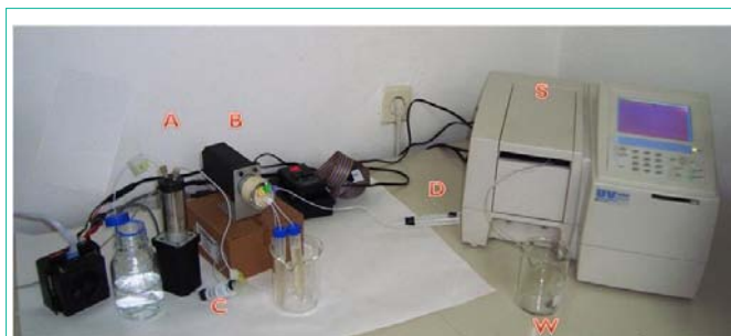
Figure 1: Sequential injection system. A-Syringe pump, B-Selection valve, C-holding coil, D-reaction coil; S-UV-Vis Spectrophotometer with flow cell ( V = 80 \mu\text{L} ), W- waste.
