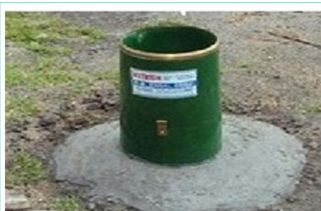
Figure 2: Rain gauge used for measuring the rainfall (mm) received during the experimental season.
