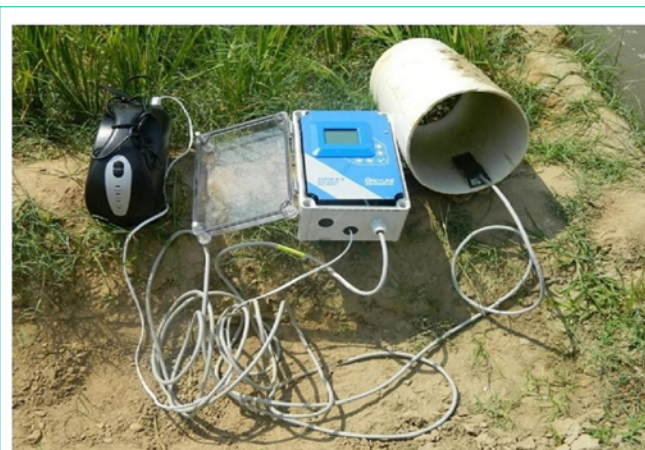
Figure 1: Complete set of flow meter with sensor in the pipe and battery for functioning of meter.
